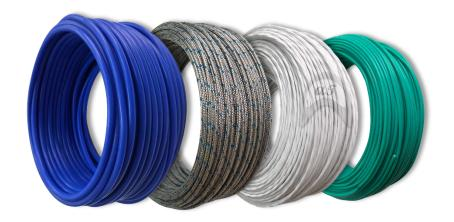
**Thermocouple / RTD Wire** is to connects the point of sensing to the point of cold junction compensation (CJC end) where the signal is measured. Thermocouple is a temperature sensor made up of two dissimilar metals that are joined together at the sensing end. Different metal mixtures in the wire are design for different thermocouple types (J, K, T, E, and so on). The insulation of the thermocouple wire can be identified according to the color coded.
